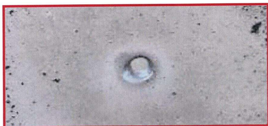
Steel thickness: 5 mm. Drilling time: 22÷24 sec. Steel thickness: 10 mm. Drilling time 55÷60 sec.
