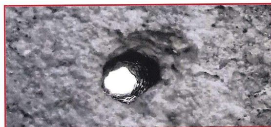
Concrete thickness: 130 mm. Drilling time: 31 sec. Cement thickness: 210 mm. Drilling time: 1 min. e 10/20 sec.
