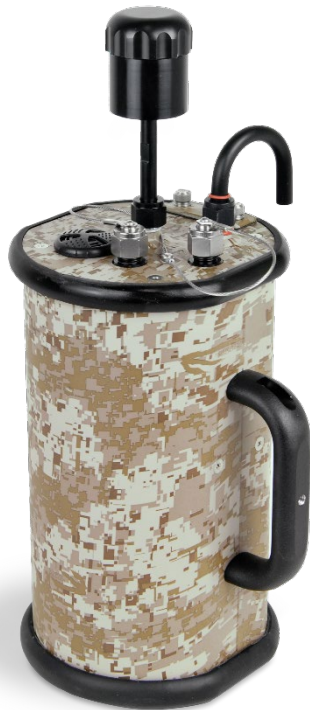
The Tac-7C ® UV-based biodetector
